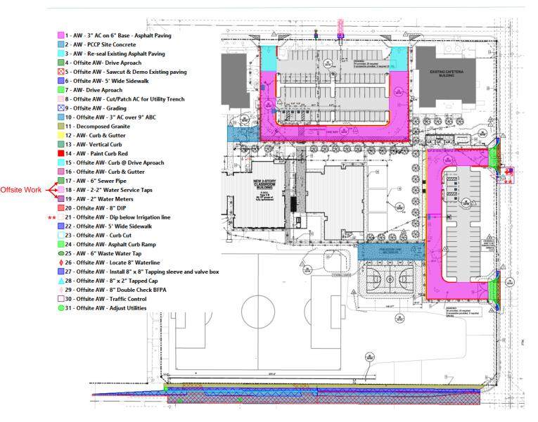
\*\* Line 21 clarification: A Back Tap is required to have the valve installed out of the sidewalk, curb, and gutter area. There is not enough separation between existing waterline and irrigation line to DIP new tap per COP Standard Detail P1370. Cannot depict by drawing
